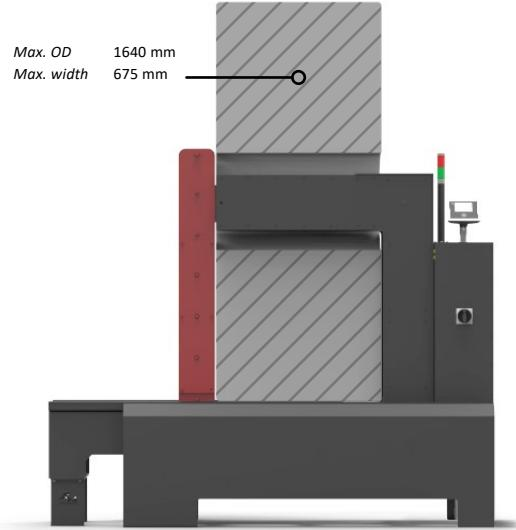
All extreme dimensions shown are theoretical. In practice there are multiple factors (e.g. workpiece weight, material and placement) that affect and limit the effective and proper heating of the workpiece.
