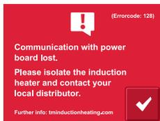
Fatal errors cannot be resolved without contacting the local distributor, as the problem is caused by an internal hardware or software error. When encountering a Fatal error the user must note the Error-code (found in the top righthand corner) and the operating conditions. Operating conditions may contain a description of the part that has been heated, the heating mode that has been used, and any other relevant information.
